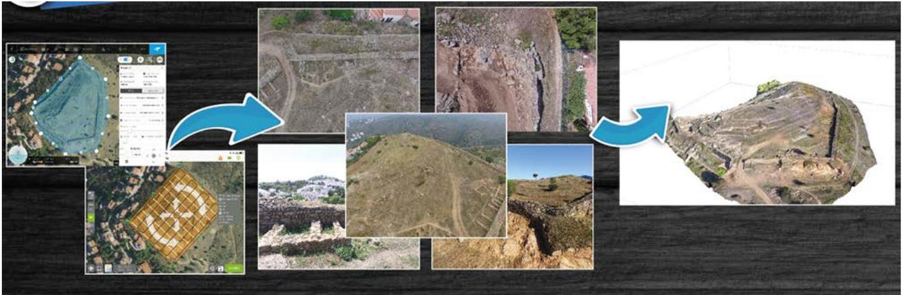
**Figure 8.** Scheme of geometric documentation through the use of drones. On the left, we can see the interfaces of the apps used to plan the flights. In the centre are the images obtained, and on the right, the resulting 3D model on which we carried out the tests and analysis.
