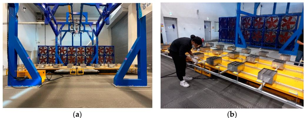
**Figure 4.** (a) Indoor simulator for UAV sprayer using artificial climate; (b) utilizing the WSP layout to evaluate spray.
