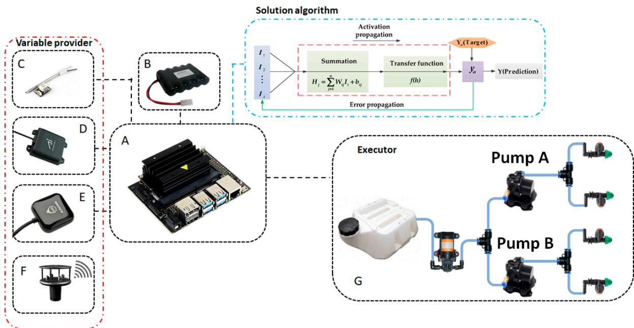
**Figure 10.** Expected independent control system, including: A. Jetson nano (main core), B. battery, C. digital airspeed sensor, D. altimeter, E. GPS, F. wind-factor sensor, G. spraying system (execution device), employing solution logic as an algorithm.
