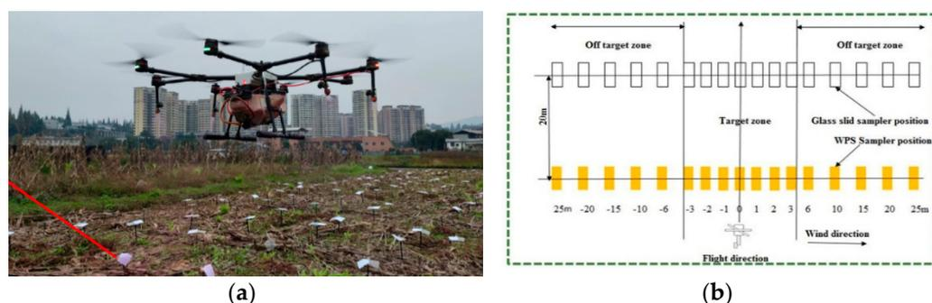
**Figure 5.** Simulator experiment schematic diagram: (a) sample data acquisition site and (b) sample data collection sketch map.
