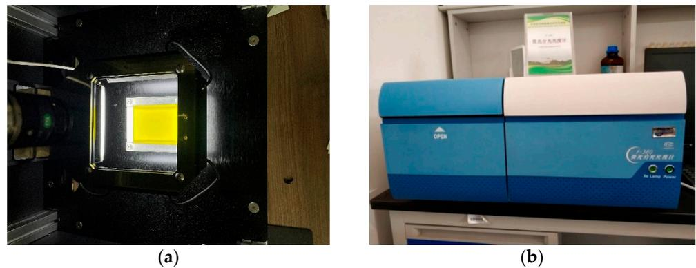
**Figure 6.** Detecting spray deposit and pattern: (a) image processing of WSP, using (b) fluorescence spectrophotometer.
