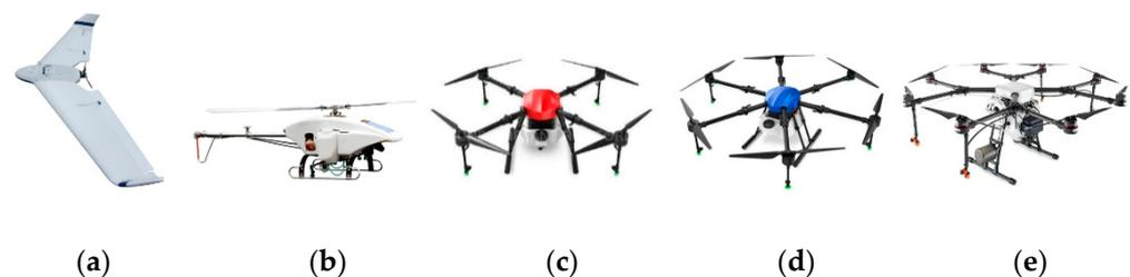
**Figure 1.** Different types of UAV: (a) Fixed Wing, (b) Single rotor, (c) Quadcopter (d) Hexacopter, and (e) Octocopter.
