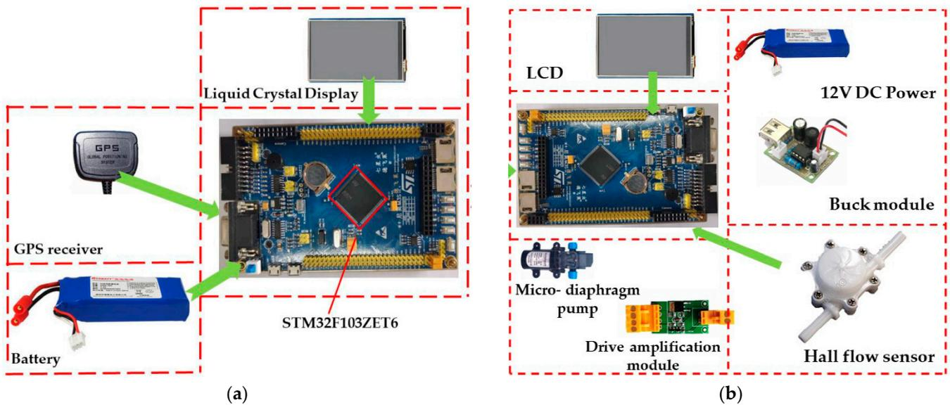
**Figure 14.** A hardware schematic depicting a prescription graphic translation system (a) and a variable spray controller (b).
