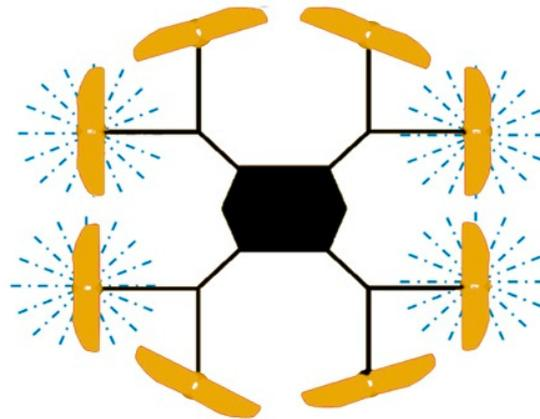
**Figure 3.** The schematic of DJI Agras MG-1 showing the rotor configurations and corresponding nozzle locations under the rotor.
