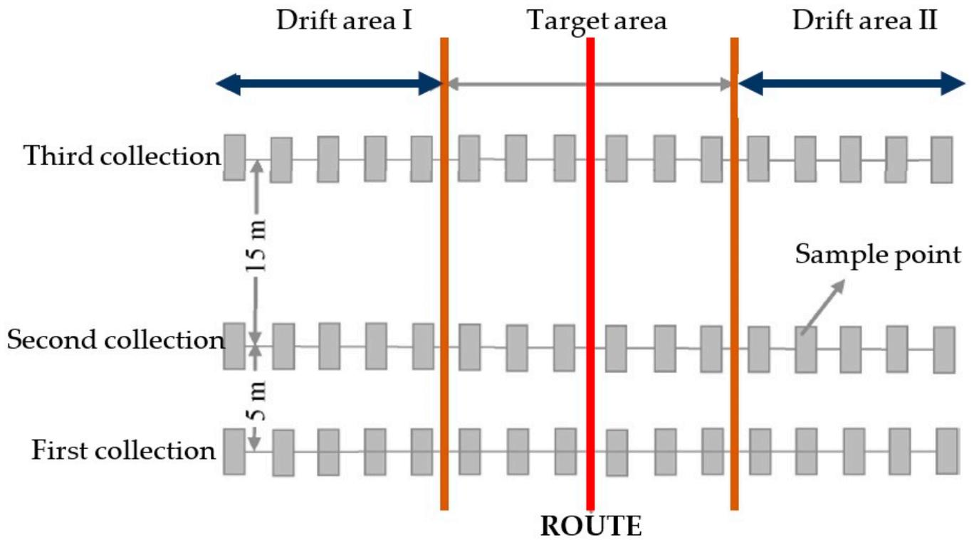
**Figure 12.** Spraying distribution schematic for the study of the effect of negative factors on UAV performance.
