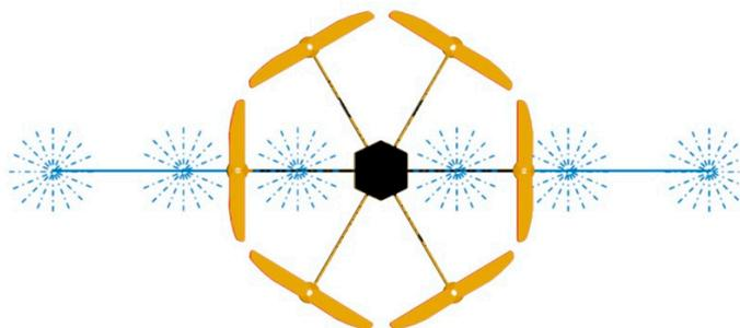
**Figure 2.** Schematic of HSE V6A, showing rotor configurations and corresponding nozzle locations on spray boom.
