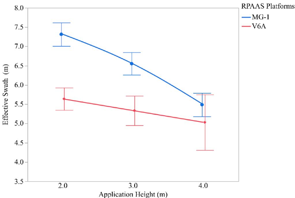
Figure 9. The effect of spraying altitudes on spray pattern uniformity by two types of drone sprayers.
