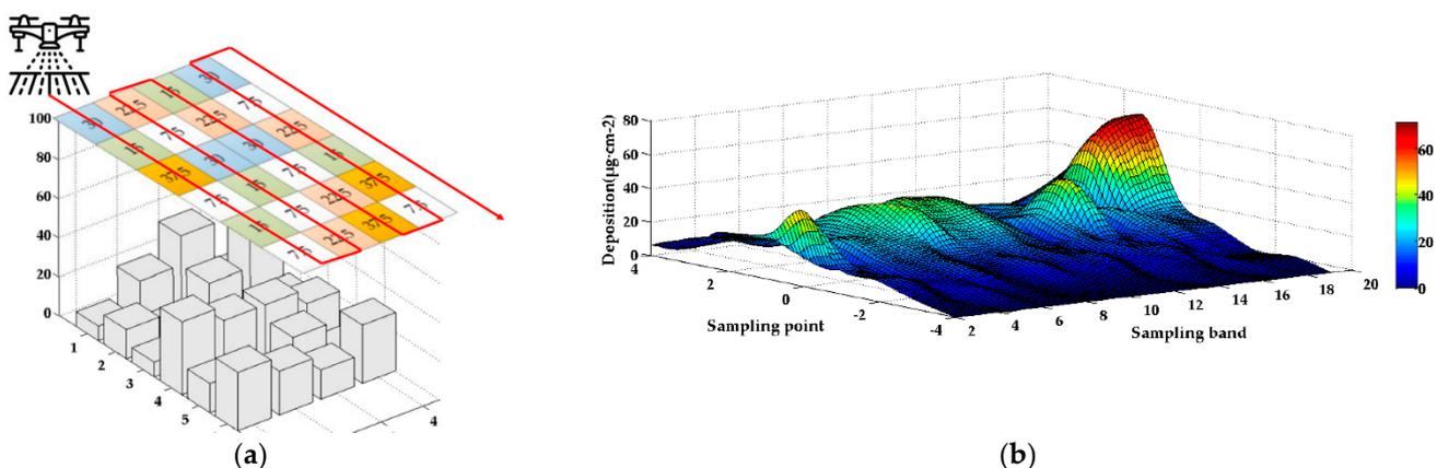
Figure 17. Comparison of reference data (a) and spray execution data (b) to identify which errors are caused by drifting.
