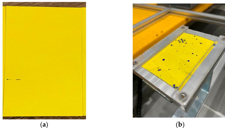
**Figure 7.** Water-sensitive paper (a) before exposure and (b) after exposure to the spray.
