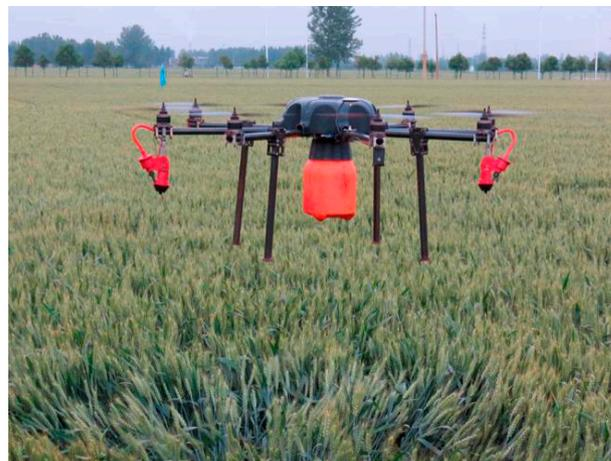
**Figure 15.** 3WTXC8-5 six-rotor UAV sprayer (Henan Tianxiucaï Aviation protection machinery Co., Ltd., Kaifeng, China).
