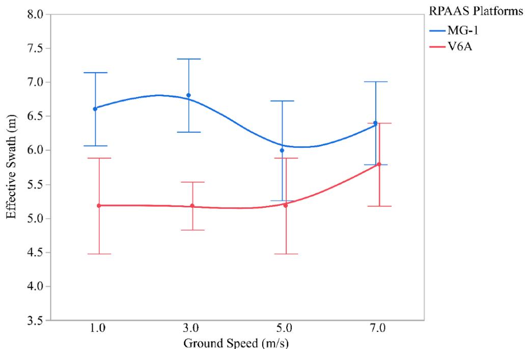
Figure 8. The effect of flying speed on spray pattern uniformity based on the two types of drone sprayers.
