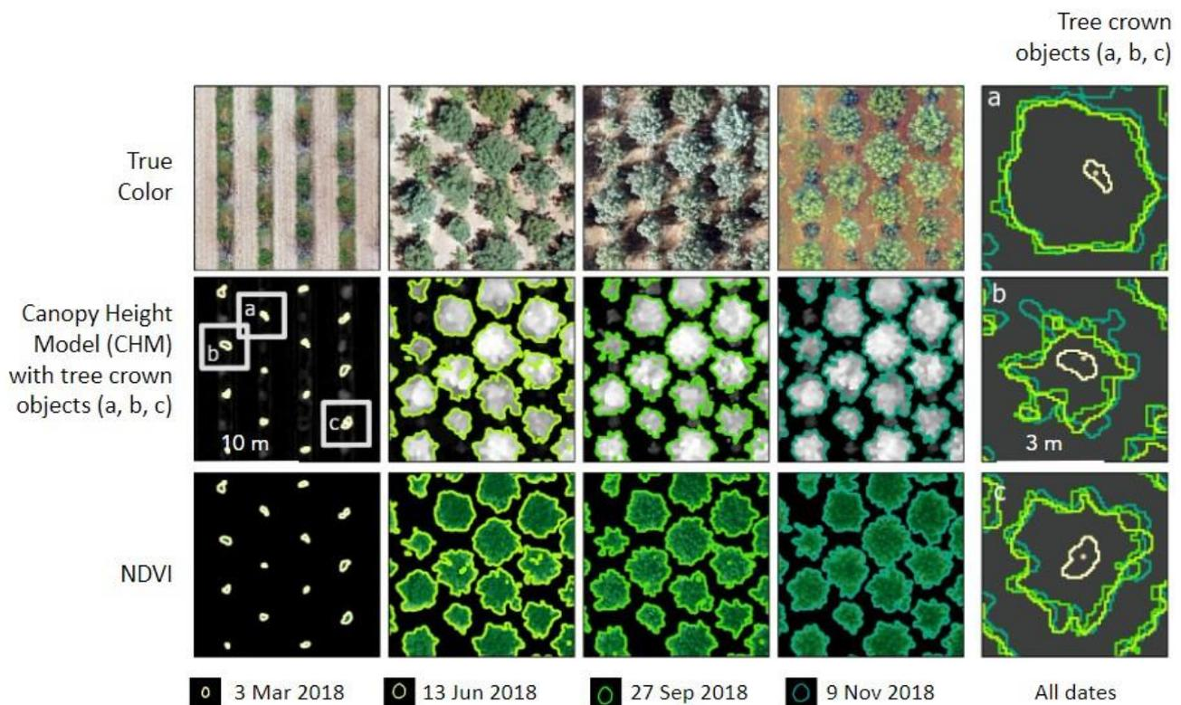
**Figure 3.** The same non-grafted UCB-1 trees in the experimental orchard. Top row: UAV-derived True Color; middle row: Canopy Height Model (CHM) (higher values are in lighter tones); bottom row: NDVI for March, June, September, and November 2018. Boxes (a–c) show the tree crown object perimeters of three individual trees throughout the growing season.
