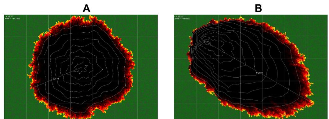
**Figure 7.** Typical outcome of a simulation run in the symmetrical (A) and biased propagation (B) scenarios (the white dot marks the point of origin). The furthest reach of the fire, the time it took for it to reach the edge of the arena and the total area destroyed up to that time are recorded. The elevation curves indicate progression and are 2' apart.
