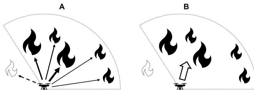
**Figure 3.** Calculation of the resultant vector. All detected heat sources are added up, taking into account range and fire intensity (A). The nearby source outside the cone of vision (west-northwest) is not included. The resultant vector points into the average direction (B).
