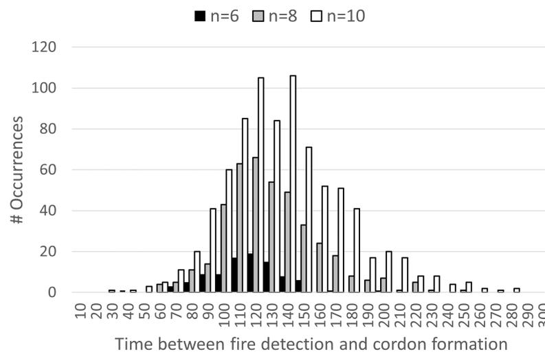
**Figure 10.** The Frequency distribution of successful encirclements as a function of the interval between locating a fire and establishing a perimeter, for three different swarm sizes ( $n = 6, 8$  and  $10$ ), operating in the largest arena ( $\approx 831$  ha). Results are for the symmetrical fire propagation scenario.
