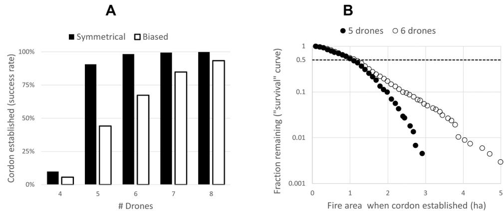
**Figure 8.** Simulation results (1000 independent realisations per combination of parameter values). (A): comparison between symmetrical and biased fire propagation. (B): “survival” curve representation of the size (surface area) of the blaze when it was successfully encircled, in the biased propagation case.
