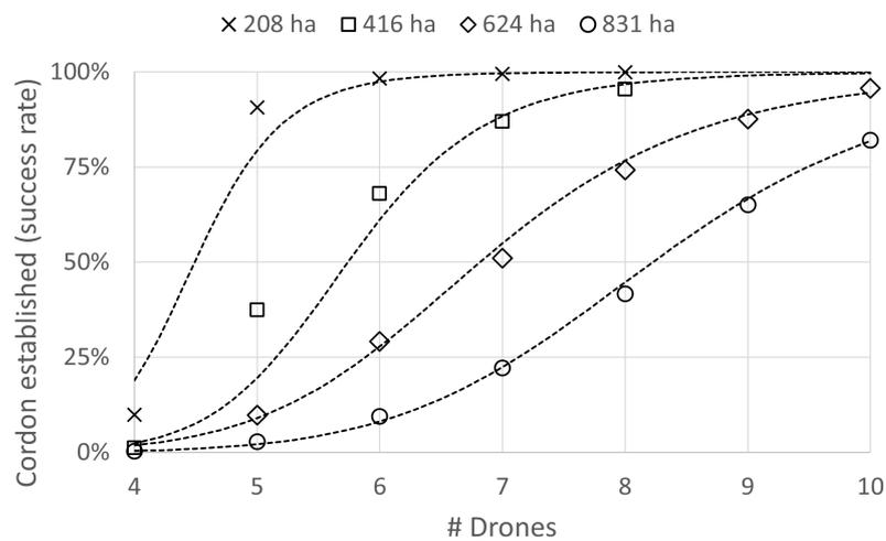
**Figure 9.** Performance evaluation for variable arena and swarm sizes. Every data point is the fraction of simulation runs that resulted in a successful perimeter being established, out of 1000 independent realisations (symmetrical fire propagation scenario).
