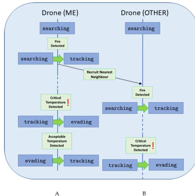
**Figure 5.** The changes in behaviour when locating a fire (by the device itself, **A** or by a neighbouring drone, **B**). Once a device is in tracking mode, it can only change into evading mode if its ambient temperatures get too hot. Once an acceptable safety distance has been reached, a drone will automatically revert to the tracking behaviour until the mission is completed.
