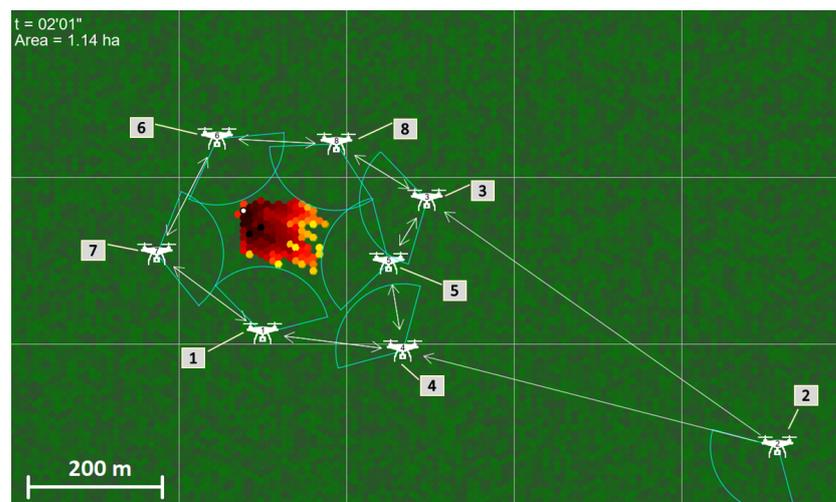
**Figure 6.** Example of a successfully established perimeter. The arrows point to the two nearest neighbours of every UAV. For a symmetrical cordon to be created, all the connections between its members must be bidirectional. This is the case here for the set containing drones 8,3,5,4,1,7,6 (2, whose nearest neighbours are 3 and 4 but is not one of theirs, is not included).
