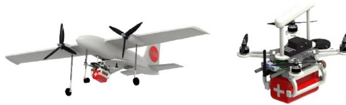
**Figure 19.** Fixed-wing UAV docking station with the multirotor UAV locking system [78]. The figure shows the concept CAD design of the fixed-wing UAV and the multirotor UAV with the docking mechanism mounted on.
