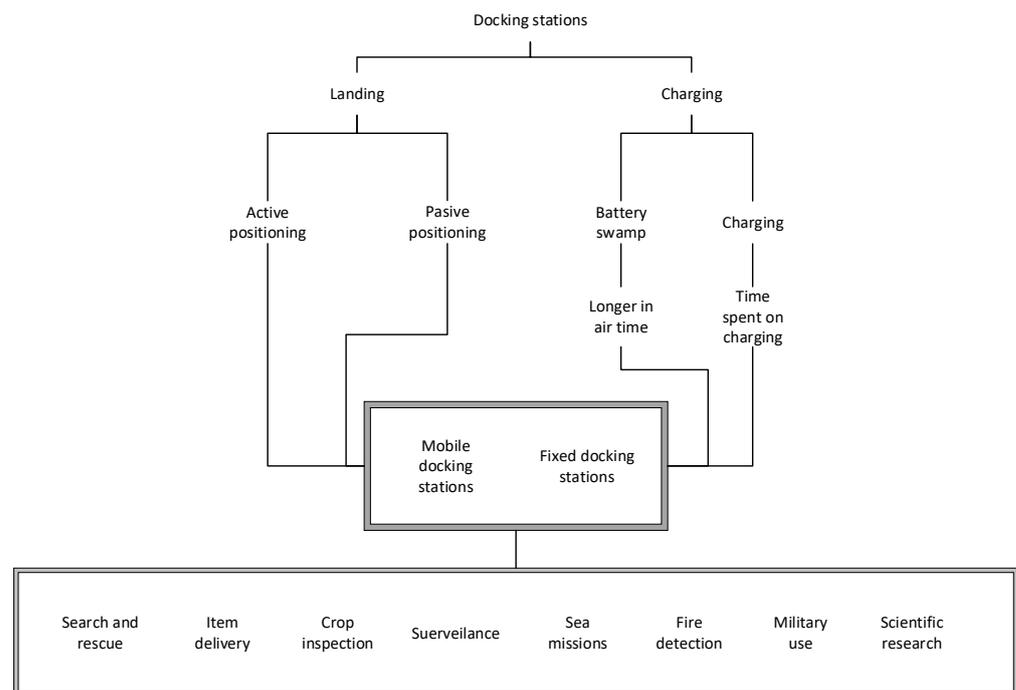
**Figure 21.** Combinations of properties and possible applications of different docking station systems.
