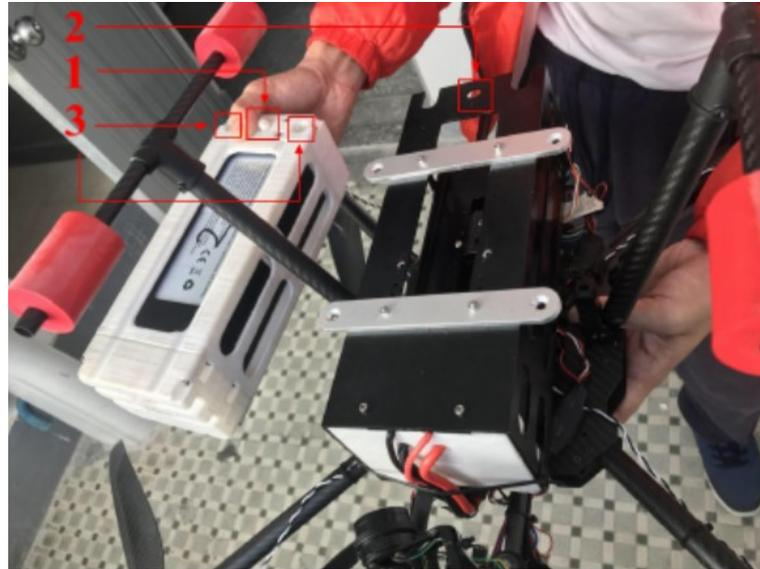
**Figure 6.** Battery compartment and the battery slot on the UAV [39]. Label 1 and 2 on the figure show the positioning system which is composed of a pin (1) that pops out to be locked in the hole (2). The two holes (3) on the battery compartment are used to push the battery compartment out.
