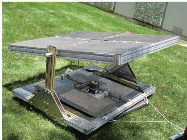
**Figure 9.** ISLANDS [28], assembled docking station with actively tilted landing pad.
