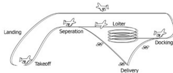
**Figure 20.** Operation concept of the proposed fixed-wing and multirotor UAV cooperation system from [78].
