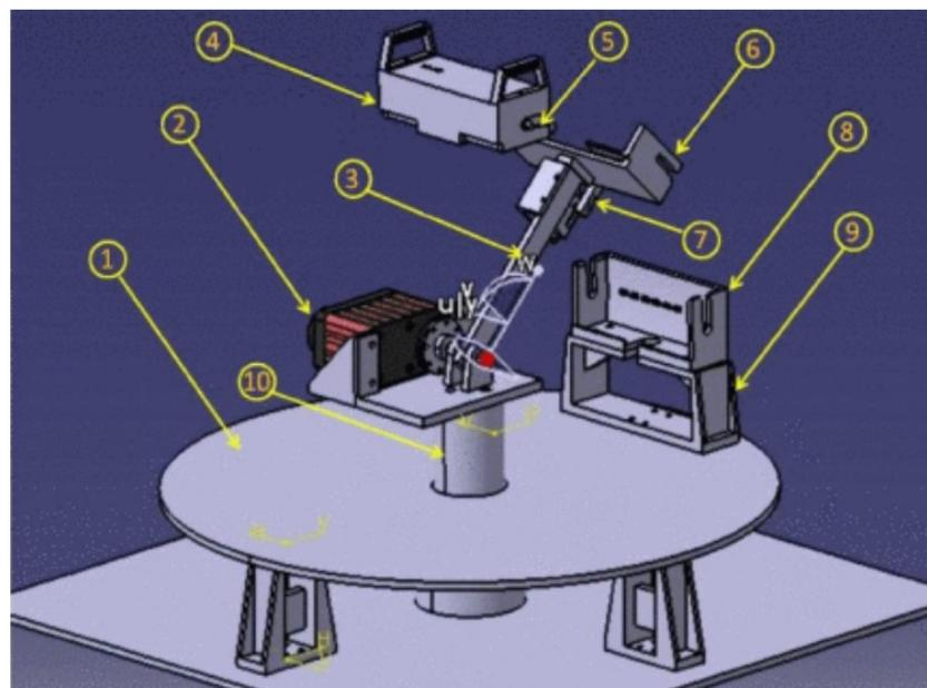
**Figure 7.** Robot arm for battery pack manipulation in [40]. The different parts are described in the paper as: Carousel (1), Servo Motor (2), Rocker Arm (3), UAV Battery Holder (4), Battery Bracket (5), Arm Battery Holder (6), Finger with motor (7), Bottom Battery Holder (8), Carousel Bracket Height (9), and Shaft (10).
