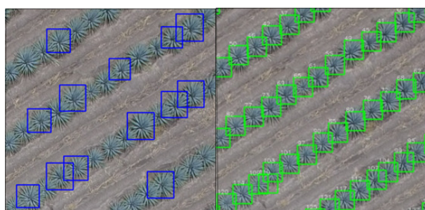
Figure 16. Comparison of the Haar classifier (left) vs. the proposed method (right).
