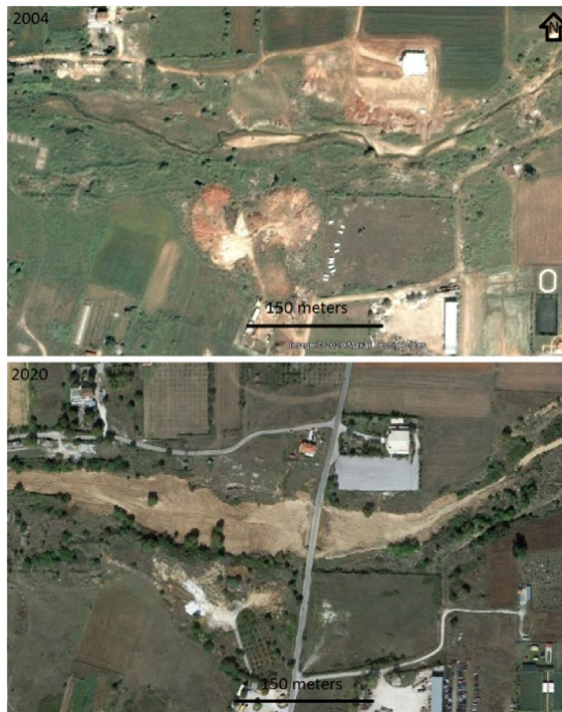
Figure 3. Google images illustrating the alteration of Kallifytos torrent due to the increase of urban infrastructure and intervention in the torrent and entire area. The images are from 2004 (top photo) and 2020 (bottom photo) (Source: Google Earth).
