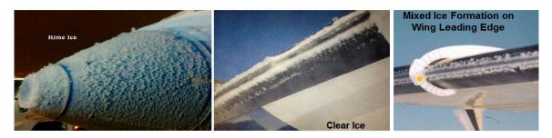
Figure 1. Ice types: rime ice, clear ice, and mixed-ice. (Photo credit: NASA, adapted from [8]).
