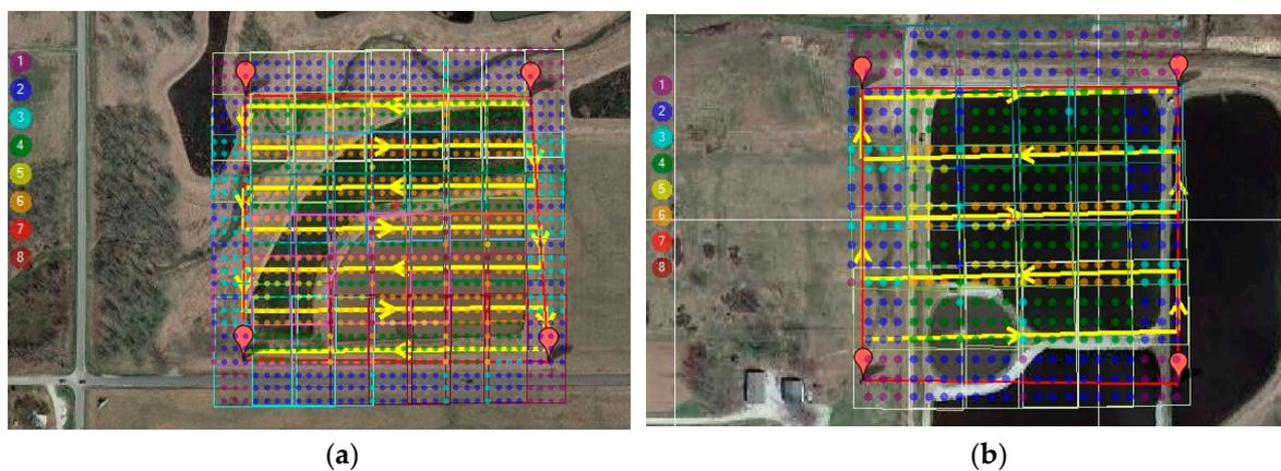
**Figure 3.** Small unmanned aerial system (sUAS) flight path (yellow arrow) and imagery footprint (with number of overlapping pictures) at the Nursery Ponds (a) and Wastewater Lagoon (b).
