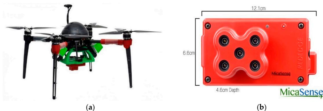
**Figure 2.** Small unnamed aerial system used to collect multispectral data (a) and MicaSense RedEdge multispectral sensor (b).
