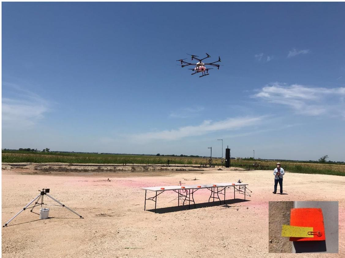
**Figure 3.** Experimental design of the study conducted over a caliche surface showing the MG-1 aircraft flying over a cotton string strung between two tripods and WSP samplers attached to five wooden blocks placed on two tables contiguous to each other. Close up of a wooden block and a WSP sampler are shown in the inset.
