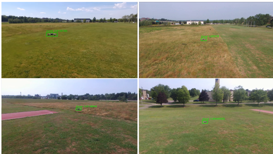
Figure 13. Examples of UAV detection in outdoor tests.
