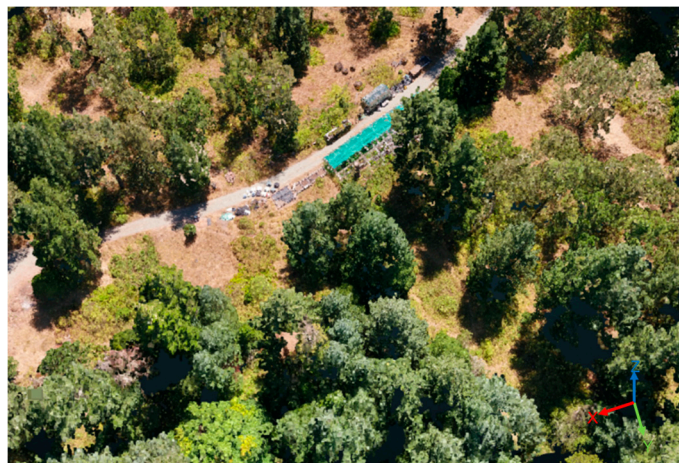
Figure 14. A subset of the SfM-MVS dense 3D point cloud (GSD = 1.28 cm) for the CGOP Meadows flight line. The Spectralon™, Flexispec™ and Permafect™ panels can be seen in the center of the path, which is the most open area in the flight line. The interactive version of the point cloud can be viewed at the following link: http://bit.ly/CGOP-MD .
