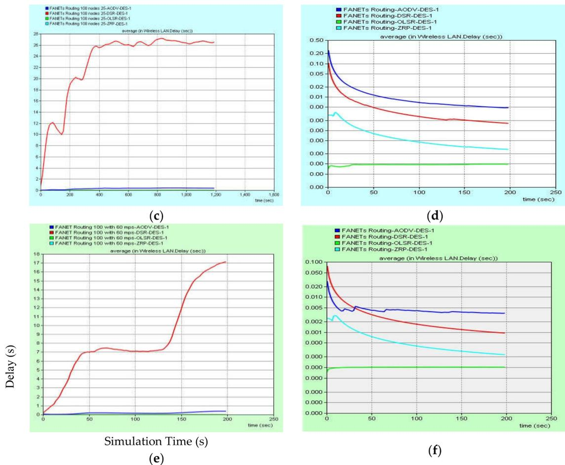
**Figure 5.** Delay simulation results (a) 30 nodes with 25 m/s and 2 km × 2 km speed and area, respectively; (b) 30 nodes with 60 m/s and 2 km × 2 km speed and area, respectively; (c) 100 nodes with 25 m/s and 2 km × 2 km speed and area, respectively; (d) 100 nodes with 25 m/s and 1 km × 1 km speed and area, respectively; (e) 100 nodes with 60 m/s and 2 km × 2 km speed and area, respectively; (f) 100 nodes with 60 m/s and 1 km × 1 km speed and area, respectively.
