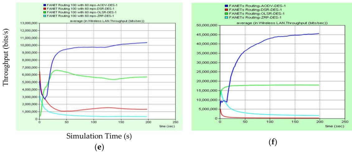
**Figure 4.** Throughput simulation results (a) 30 nodes with 25 m/s and 2 km × 2 km speed and area, respectively; (b) 30 nodes with 60 m/s and 2 km × 2 km speed and area, respectively; (c) 100 nodes with 25 m/s and 2 km × 2 km speed and area, respectively; (d) 100 nodes with 25 m/s and 1 km × 1 km speed and area, respectively; (e) 100 nodes with 60 m/s and 2 km × 2 km speed and area, respectively; (f) 100 nodes with 60 m/s and 1 km × 1 km speed and area, respectively.
