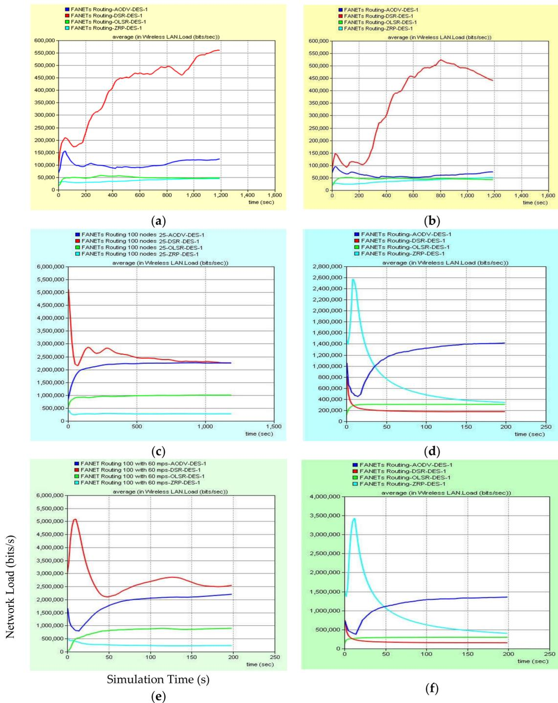
**Figure 6.** Network load simulation results (a) 30 nodes with 25 m/s and 2 km × 2 km speed and area, respectively; (b) 30 nodes with 60 m/s and 2 km × 2 km speed and area, respectively; (c) 100 nodes with 25 m/s and 2 km × 2 km speed and area, respectively; (d) 100 nodes with 25 m/s and 1 km × 1 km speed and area, respectively; (e) 100 nodes with 60 m/s and 2 km × 2 km speed and area, respectively; (f) 100 nodes with 60 m/s and 1 km × 1 km speed and area, respectively.
