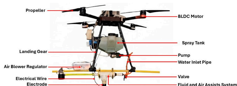
Figure 2. Components of a drone-based air-assisted electrostatic spraying system.
