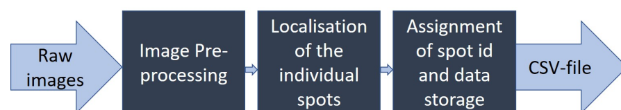
Figure 7. A flowchart illustrating the signal processing sequence applied to the 30 calibration images.
