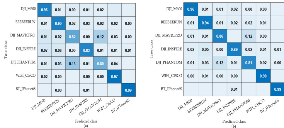
Figure 7. Confusion matrices of UAV classification at 10 dB SNR: (a) Without feature selection; (b) With feature selection.
