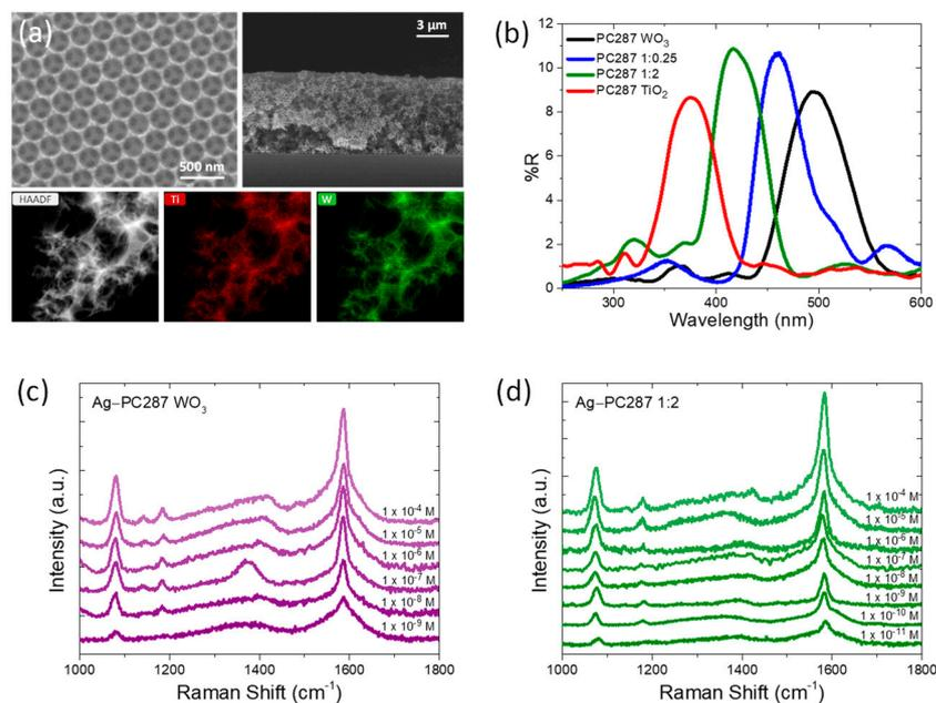
**Figure 1.** (a) (Upper) Top view and cross-section SEM images and (Lower) TEM image and elemental EDX maps of Ti and W for PC287 1:0.25; (b) specular reflectance (R%) spectra for PC287 films; (c,d) SERS spectra of 4-MBA on Ag-PC287 WO<sub>3</sub> and 1:2 substrates.
