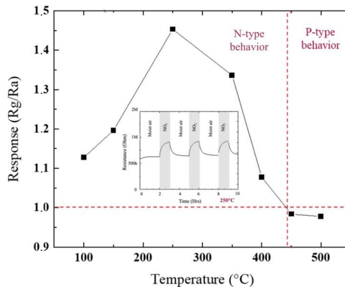
Figure 3.  $\text{NO}_2$ -sensing performance.
