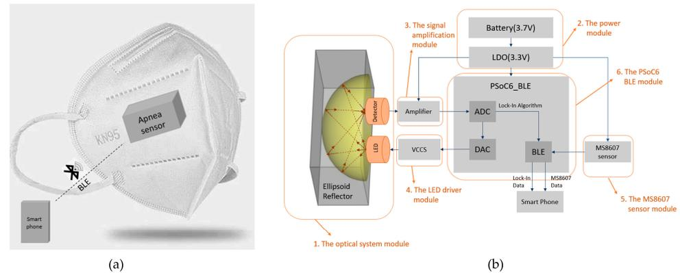
**Figure 1.** (a) Schematic overview of the wireless, embedded system design for apnea diagnosis. (b) The system concept including a highly selective, miniaturized CO<sub>2</sub> sensing module.
