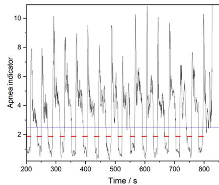
**Figure 2.** The real time values of the apnea indicator (black line) during a laboratory test and simulated apnea events. The system's algorithm reliably detected patterns in line with OSA. The blue line represents the threshold value under which an apnea episode is detected, the red lines are time intervals in which a simulated apnea event occurred.
