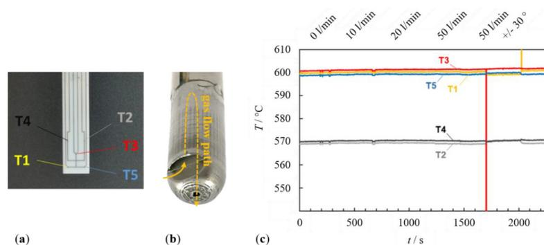
**Figure 1.** Example of a verification measurement: Sensor transducer (a) with screen-printed Pt-Au-thermocouples protected by individual modelled and additive-manufactured cap (b). Temperature characteristics on the sensors surface were measured under varying gas flows (c). The temperatures were even unaffected by twisting the sensor orientation.
