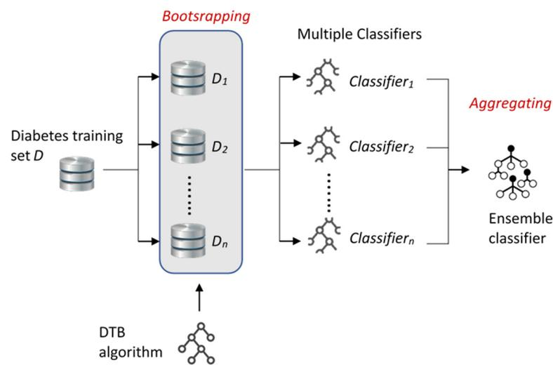
**Figure 1.** The general structure of bagging approach in this study.
