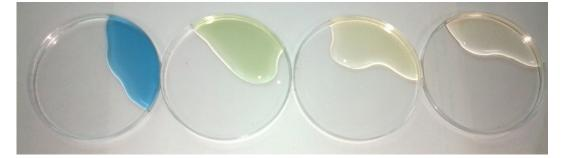
Figure 6. Decolorization of the sample solution after the different durations of Ar plasma irradiation.
