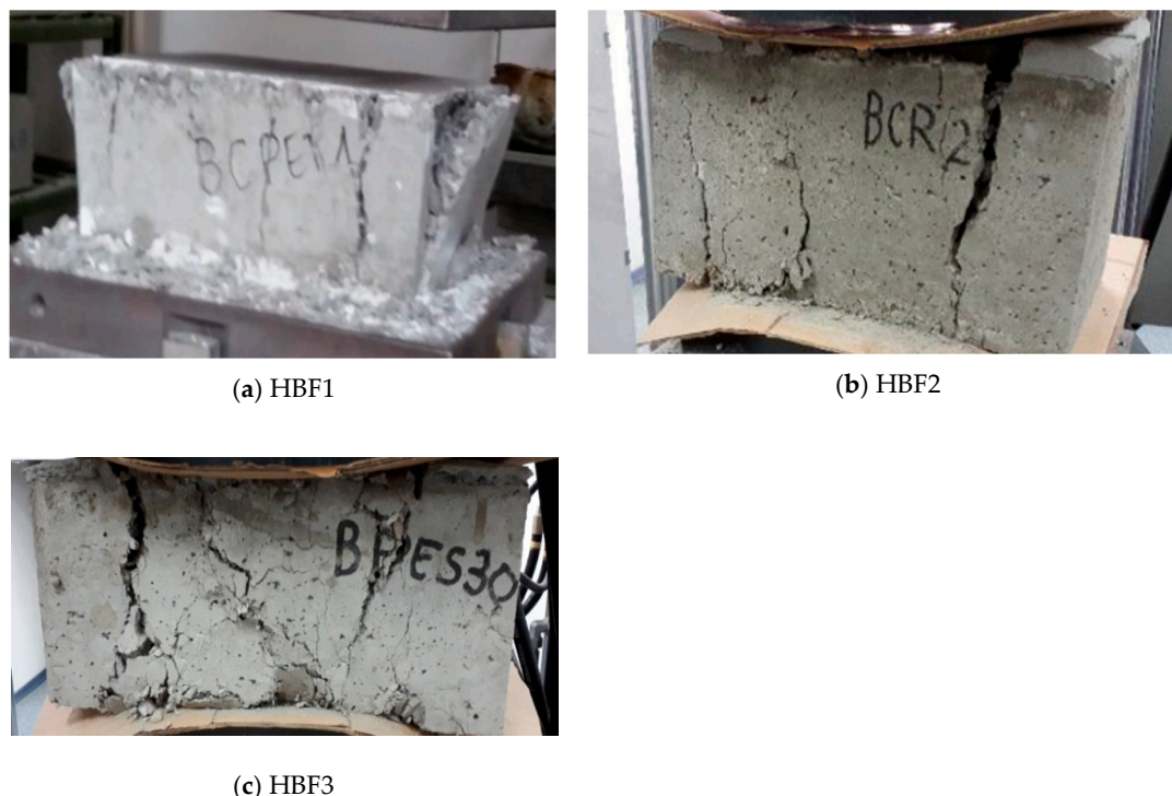
Figure 2. Failure of hollow blocks HB1, HB2 and HB3.
