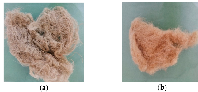
Figure 4. Retama monosperma stem fibers. (a) Before manual carding; (b) after manual carding.
