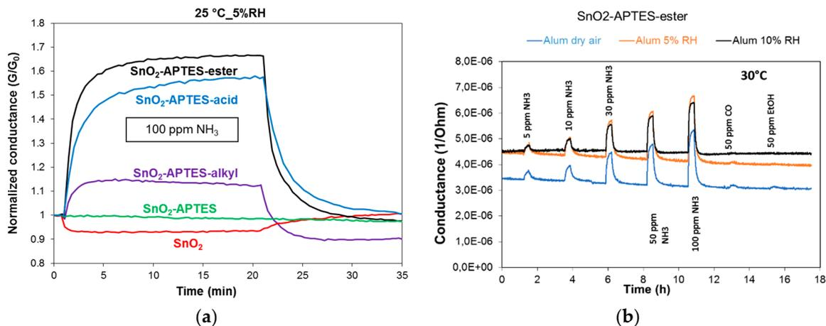
**Figure 1.** Functionalized SnO<sub>2</sub> sensor developed by screen-printing on alumina substrate: (a) Influence of end functional group on 100 ppm NH<sub>3</sub> normalized response (G/G<sub>0</sub> ratio conductance under gaz/air), at 25 °C, 5% relative humidity (RH); (b) Selective responses of SnO<sub>2</sub>-APTES-Ester to NH<sub>3</sub> and influence of humidity at 30 °C.
