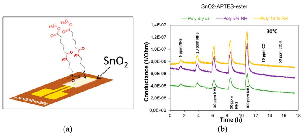
**Figure 2.** Functionalized SnO<sub>2</sub> sensor developed by inkjet on polyimide substrate: (a) schematic view of flexible sensor on polyimide with ester functionalized layer (b) Selective responses to NH<sub>3</sub> and influence of humidity at 30 °C.
