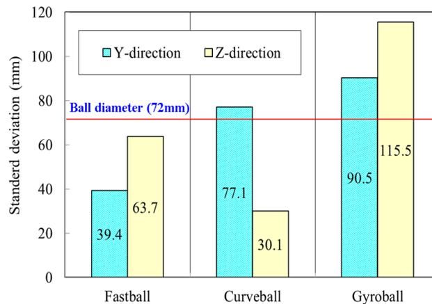
**Figure 8.** The standard deviations of the position error in each of the three pitch types. The errors of the fastball and curveball are approximately the diameter of one baseball, and the error of gyroball is less than 1.5 times the diameter of a baseball.
