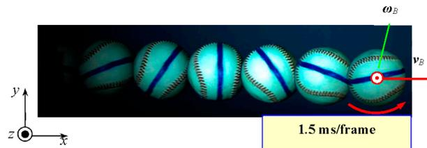
**Figure 5.** Stroboscopic image of a baseball thrown as a fastball. The ball speed  $V$  is 161 km/h and the rotation of the ball is a back spin. The ball spin rate  $S$  is 3700 rpm, and the spinning axis of  $\omega_B$  is in the direction of the  $z$ -axis.
