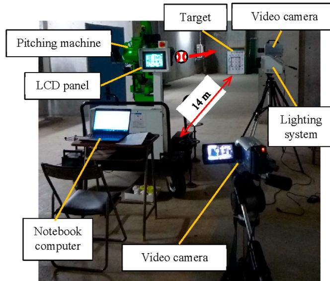
Figure 3. Setup of pitching test using the four-roller baseball pitching machine.
