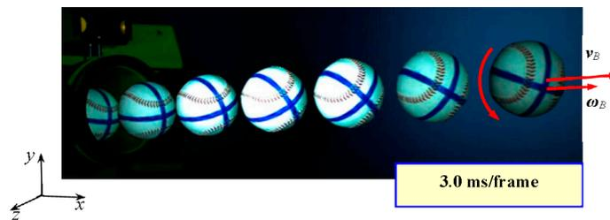
**Figure 6.** Stroboscopic image of a baseball thrown as a gyroball. The ball speed  $V$  is 105 km/h and the rotation of the ball is a gyro spin. The gyro spin rate  $S$  is 800 rpm, and the spinning axis of  $\omega_B$  is nearly the same as the flight direction of  $v_B$ , which is in the direction of the  $x$ -axis.
