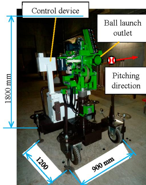
Figure 2. Prototyped four-roller baseball pitching machine.
