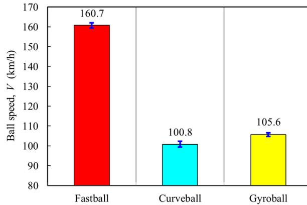
**Figure 4.** Ball speed  $V$  in three pitch types (fastball, curveball, and gyroball) using the prototyped four-roller baseball pitching machine.
