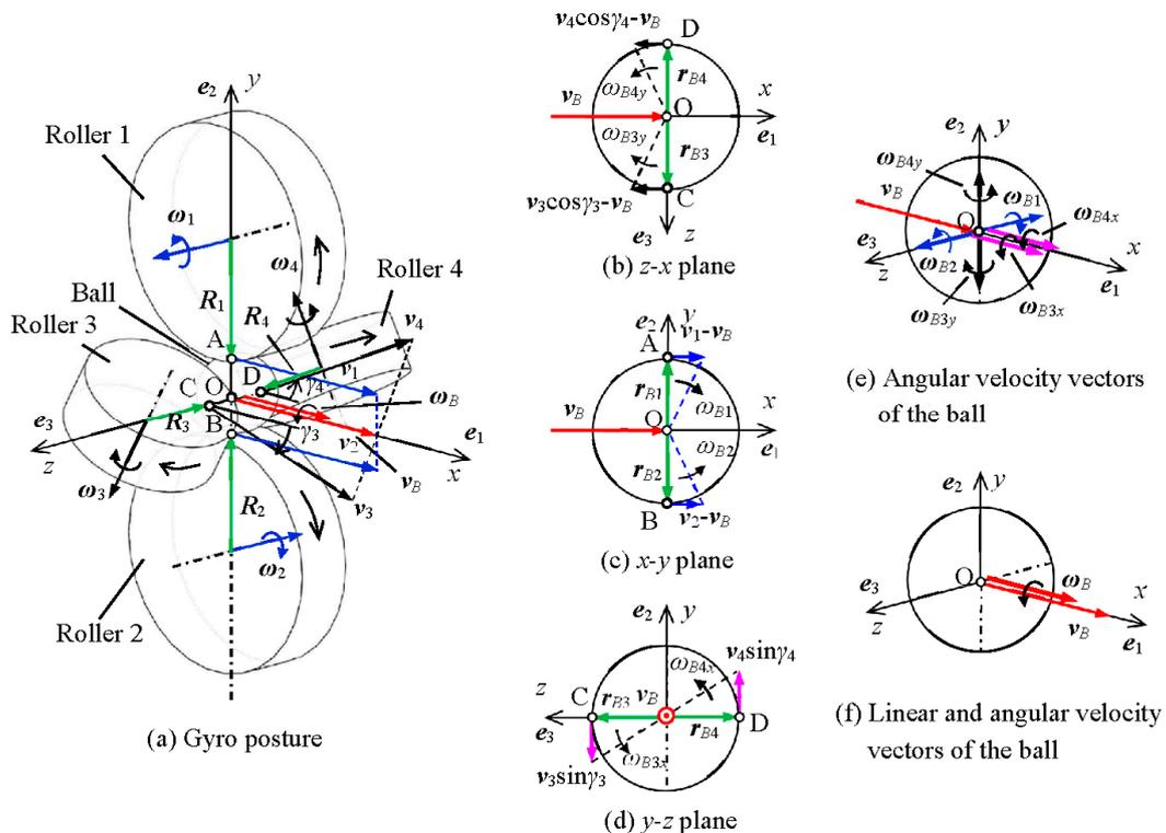
**Figure 1.** Linear and angular velocity vectors in the four-roller ball throwing mechanism by gyro posture: (a) Gyro posture; (b) z–y plane; (c) x–y plane; (d) y–z plane; (e) angular velocity vectors of the ball; (f) linear and angular velocity vectors of the ball. When the linear velocity vectors are  $v_1 = v_2 = v_3 = v_4$ , and the linear velocity vector  $v_B$  and angular velocity vector  $\omega_B$  of the ball are in the same direction, a gyroball can be thrown.
