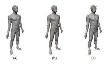
**Figure 2.** Process of individual model construction. (**a**) Import body shape data; (**b**) construct link segment model; (**c**) added feature points at the same positions as used for underwater motion-capture measurement.
