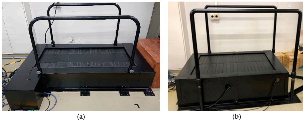
Figure 1. Two types of load-controlled treadmills: (a) single-belt style; (b) split-belt type divided into left and right.
