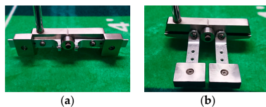
Figure 4. Adjustable putter used for physical testing. (a) Configuration A ( r_{cy} = 11.2 mm, I_{cz} = 3997 g cm 2 , m_c = 360 g); (b) Configuration B ( r_{cy} = 25.2 mm, I_{cz} = 4790 g cm 2 , m_c = 360 g).
