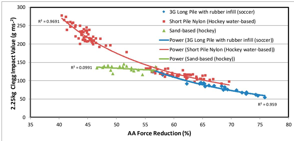
**Figure 3.** The relationship between the industry standard AAA and the 2.25 kg Clegg Hammer for three different generic types sport surface systems (modified from [1]).
