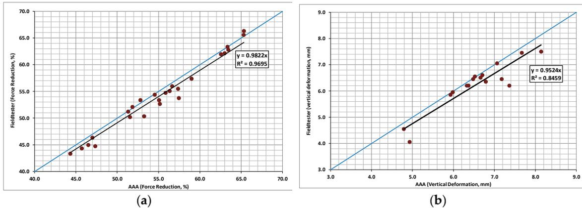
**Figure 4.** Correlations for the Fieldtester and AAA on a range of laboratory samples and field data, for force reduction (FR) (a) and vertical deformation (VD) (b). The line of equality is shown, and the best fit lines forced through the origin.
