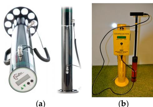
**Figure 2.** (a) the Fieldtester showing the readout unit (left) and in profile (right) (reproduced from [3]); (b) the Clegg Impact Soil Tester (2.25 kg unit) and guide tube with the readout unit attached.
