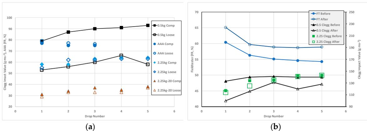
**Figure 5.** (a) Laboratory impact test data on a rubber infilled carpet for “loose” and “compacted” (Comp) states. (b) Field data (for a specific position, and typical of all positions) for 5 repeated impacts with the Fieldtester (FT) and CIST devices, showing results for “before” and “after” a deep decompaction of the infill.
