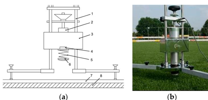
**Figure 1.** (a) schematic of the Advanced Artificial Athlete (AAA) [1]: 1. Support frame; 2. Electric magnet; 3. Falling mass; 4. Accelerometer; 5. Spring; 6. Test foot; 7. Test surface; 8. rigid floor; (b) photograph of the AAA setup.
