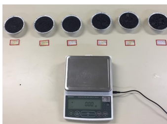
Figure 5. Verification aliquots of pellet feed standard samples after weighing and heating for 24 h at 105 °C.
