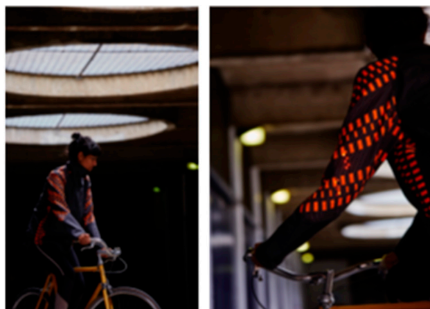
Figure 1. Light my Elbows cycling jacket incorporating LEDs within electronic yarns in the elbows.
