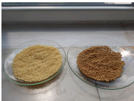
Figure 3. NPK granules before and after coating.
