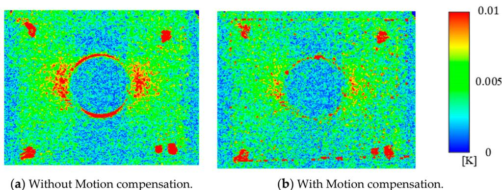
**Figure 4.** Distributions of dissipated energy ( $\sigma_a = 50$  MPa).
