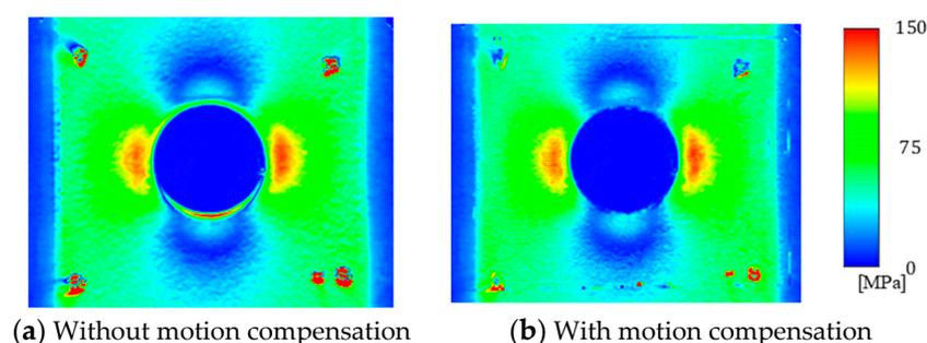
**Figure 3.** Distributions of measured stress amplitude ( $\sigma_a = 50$  MPa).
