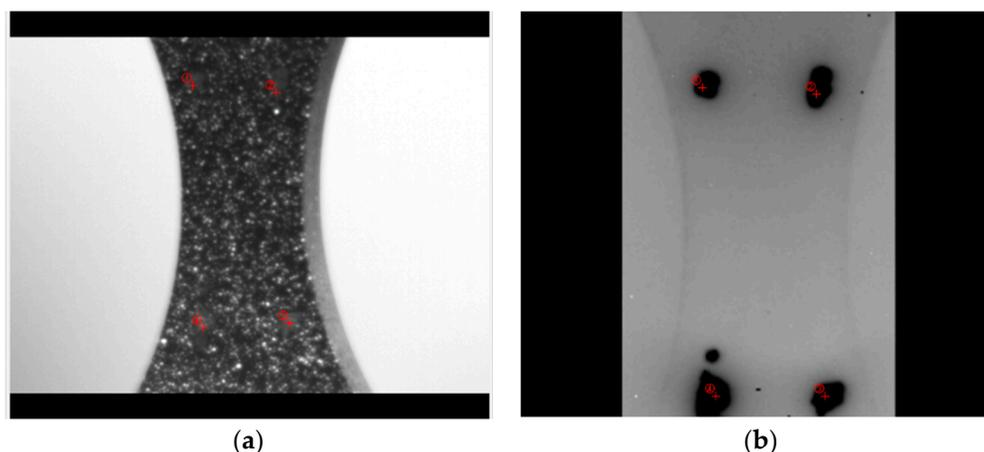
**Figure 2.** Four pairs of coordinates for obtaining a homography transformation matrix: (a) Visible image, (b) Infrared thermography.
