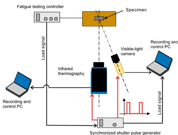
**Figure 1.** Schematic illustration of optical-infrared thermography synchronous measurement system.
