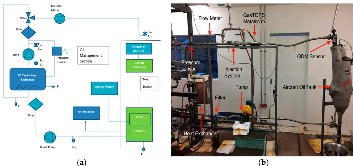
**Figure 4.** Oil test bench: (a) Hydraulic diagram of the oil test bench; (b) installation of the hydraulic circuit.
