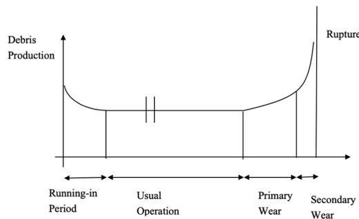
**Figure 1.** Generation rate of debris of a component in the oil lubrication system.
