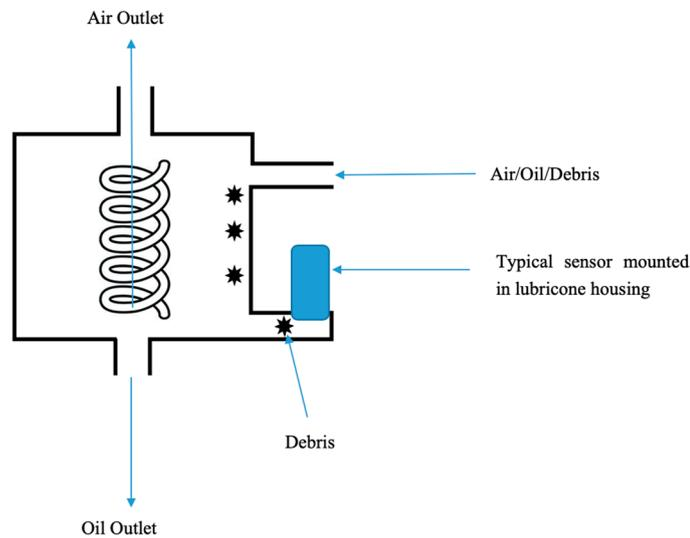
Figure 3. Vortex separator of the QDM sensor.
