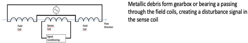
Figure 2. The three field coils.
