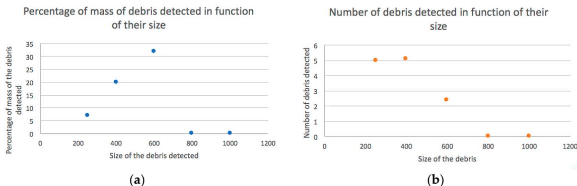
**Figure 6.** Test Package 2: (a) Average amount of debris detected as a function of size by the GasTOPS sensor; (b) percentage of the average mass of debris detected as a function of size by the GasTOPS sensor.
