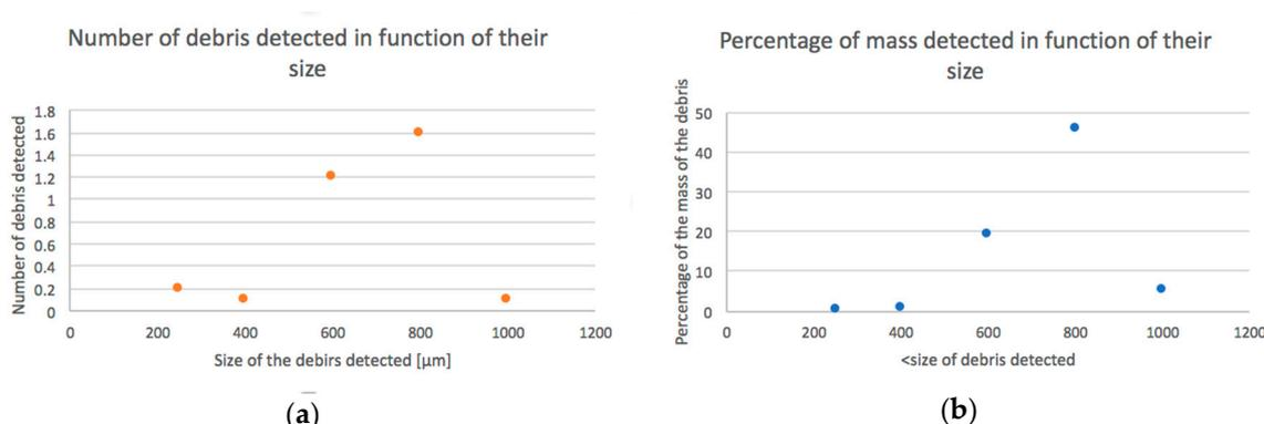
**Figure 5.** Test Package 1: (a) Average amount of debris detected as a function of size by the GasTOPS sensor; (b) percentage of the average mass of debris detected as a function of size by the GasTOPS sensor.
