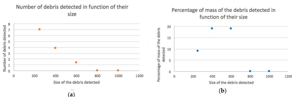
**Figure 7.** Test Package 3: (a) Average amount of debris detected as a function of the size by the GasTOPS sensor; (b) percentage of the average mass of debris detected as a function of the size by the GasTOPS sensor.
