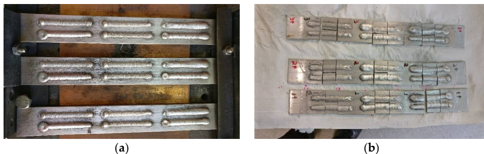
Figure 2. Aluminum specimens: (a) welding samples; (b) cut welding samples.
