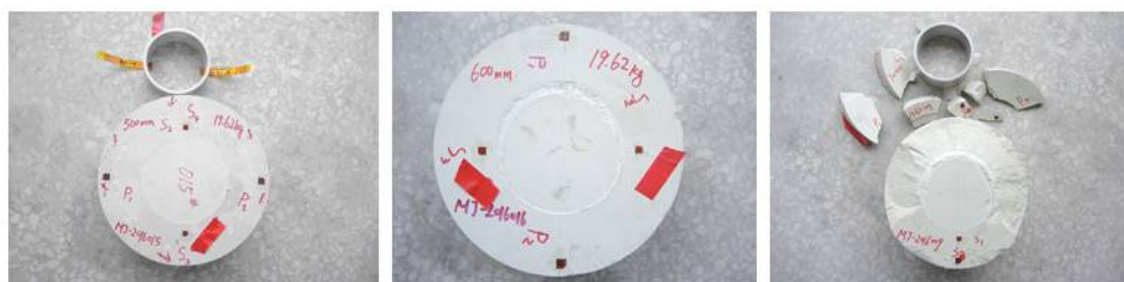
Figure 7. Morphology of PBX simulation material after drop test.
