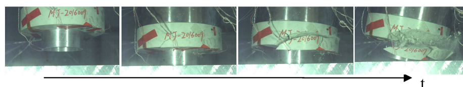
Figure 6. Drop test piece impact process.
