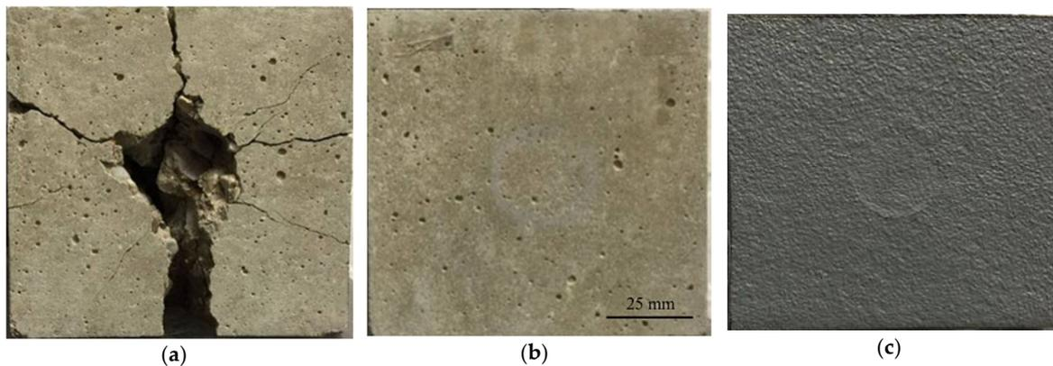
**Figure 1.** Recovered specimens after impact at 65 m/s (a) Impacted face of uncoated concrete cube; (b) Underlying concrete damage when coated with 5 mm elastomer layer; (c) Impacted face of 5 mm elastomer layer.
