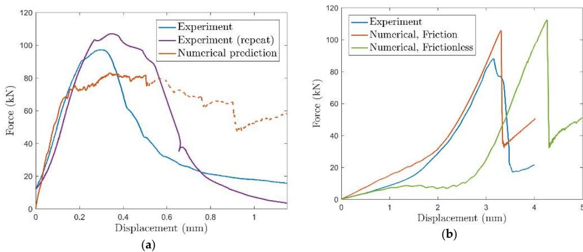
**Figure 2.** Quasi-static indentation tests on 100 mm concrete cubes (a) Uncoated concrete; (b) Concrete coated with 5 mm elastomer layer.
