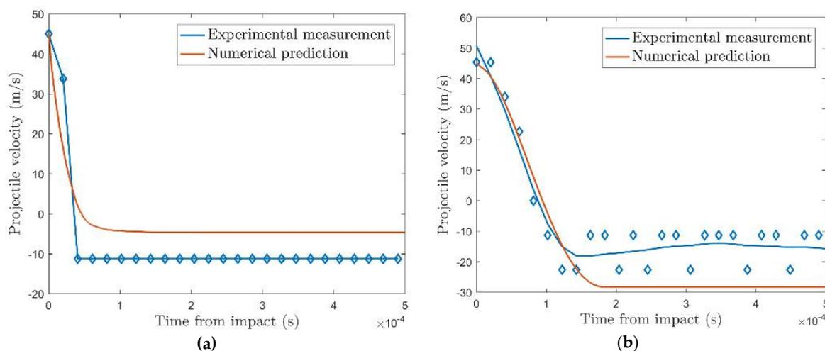
**Figure 3.** Projectile velocity-time histories for impact indentation at 45 m/s (a) Uncoated concrete cube; (b) Concrete coated with 5 mm elastomer layer. A positive velocity is defined to be in the direction of impact.
