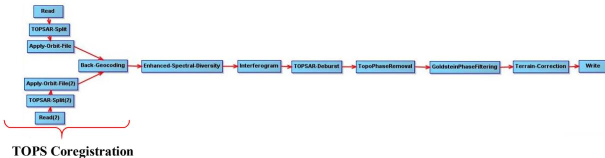
Figure 3. Flow chart of the Sentinel-1 TOPS data coregistration.
