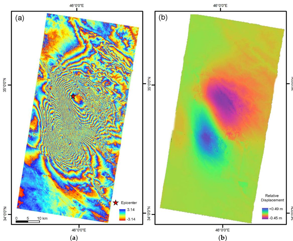
**Figure 4.** Geocoded interferogram (a), and geocoded unwrapped phase (b).
