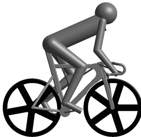
**Figure 1.** MapleSim model of a cyclist and bicycle consisting of eleven bodies with seven degrees of freedom. The head, arms, and trunk were fixed and therefore treated as a single body.
