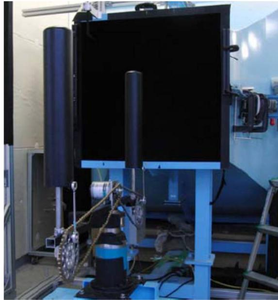
Figure 4. Two oscillating circular cylinders in a tandem arrangement.
