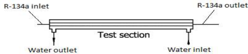
Figure 1. The schematic figure of the micro-fin tube-in-tube heat exchangers (Wongsa-ngam et al., [10]).
