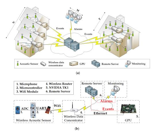
**Figure 4.** Network topology description of the proposed AAL system proposed and the technological proposal of the devices which integrate that system. (a) Network topology of the system and (b) subsystems that integrate that full system and the elements used in each subsystem.
