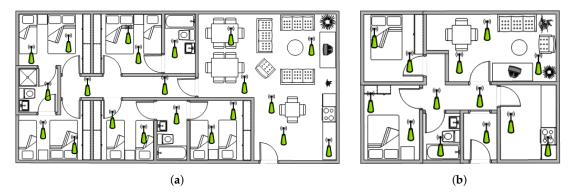
**Figure 2.** Detail of the alternative implementation of an acoustic alarm service, taking into account the sensing of all the available spaces in each type of living place. (a) Residence site, with several buildings/houses with common spaces (dining room, etc.) and with private facilities for elderly or pseudo-dependent; (b) Isolated flats where elderly or pseudo-dependent people need basic surveillance support.
