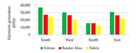
Figure 2. Electricity generation for Poly-Si for different sides.
