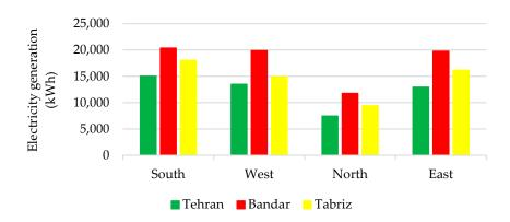
Figure 3. Electricity generation for Cd-Te for different sides.
