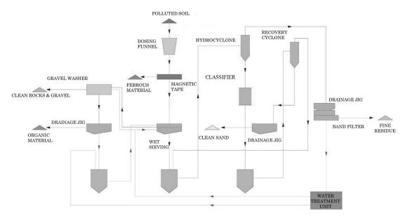
Figure 1. Scheme of a mobile plant of soil washing (Courtesy of Soldec Tecnologías Ambientales).
