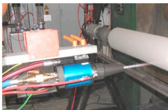
Figure 2. The process of HVOF gun deposition of composite layers. The supersonic gas jet forms the stationary shock waves in the plasma jet.
