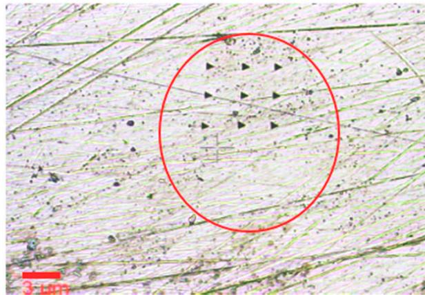
**Figure 13.** Optical imaging of the layer deposition and nano-indentation Map in hardness determination of specimen.
