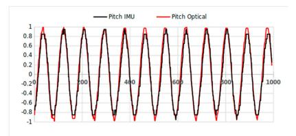
**Figure 2.** Results of using the IMU to test a Computer Vision tracking algorithm using a pendulum movement (in degrees).
