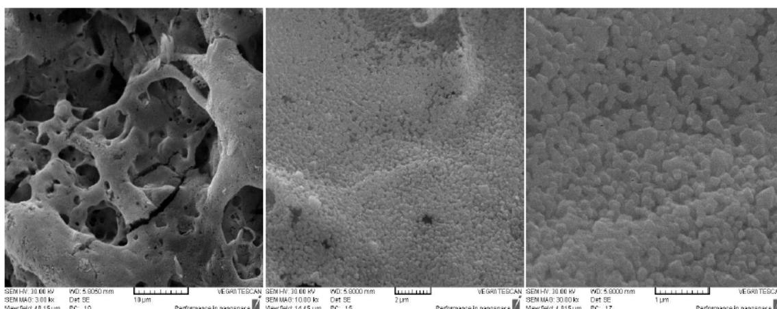
**Figure 2.** SEM images of  $\text{CuCr}_2\text{O}_4$  nanoparticles at  $850\text{ }^\circ\text{C}$ .
