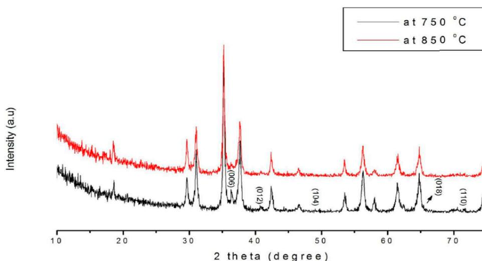
**Figure 1.** XRD patterns of  $\text{CuCr}_2\text{O}_4$  nanoparticles at 750 and 850 °C.
