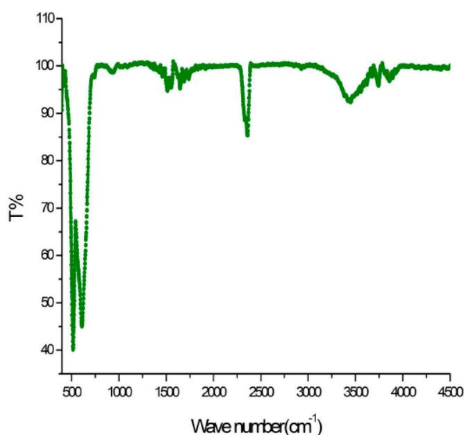
**Figure 3.** FT-IR spectrum of  $\text{CuCr}_2\text{O}_4$  nanoparticles at  $850\text{ }^\circ\text{C}$ .
