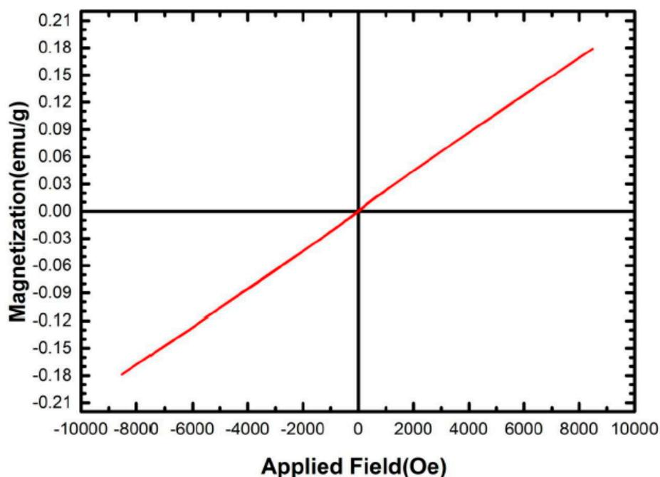
Figure 4. Hysteresis loop of CuCr<sub>2</sub>O<sub>4</sub> nanoparticles at 850 °C.
