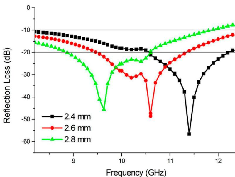
Figure 5. Microwave reflection losses of the CuCr<sub>2</sub>O<sub>4</sub>/silicone rubber nanocomposites with various thicknesses.
