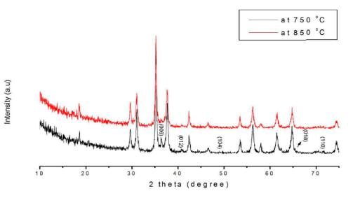
Figure 1. XRD patterns of CuCr<sub>2</sub>O<sub>4</sub> nanoparticles at 750 and 850 °C.
