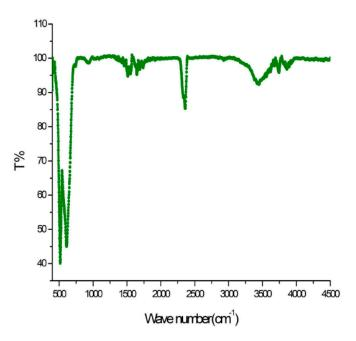
Figure 3. FT-IR spectrum of CuCr<sub>2</sub>O<sub>4</sub> nanoparticles at 850 °C.
