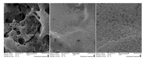
Figure 2. SEM images of CuCr<sub>2</sub>O<sub>4</sub> nanoparticles at 850 °C.
