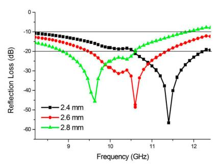
**Figure 5.** Microwave reflection losses of the CuCr<sub>2</sub>O<sub>4</sub>/silicone rubber nanocomposites with various thicknesses.
