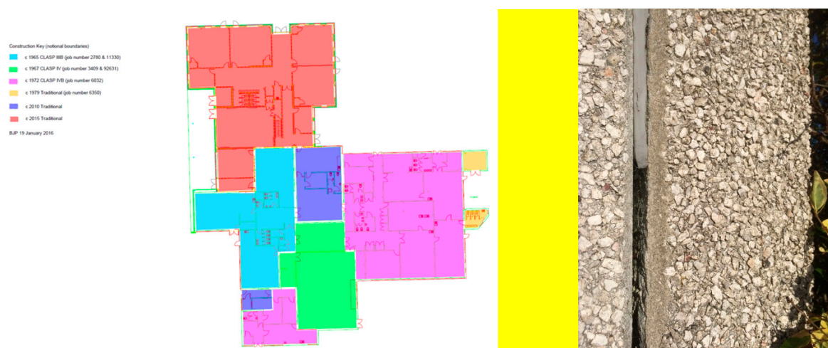
Figure 3. Plan view of UK school building and a portion of the precast skin requiring retrofit on the south façade of the plan view.
